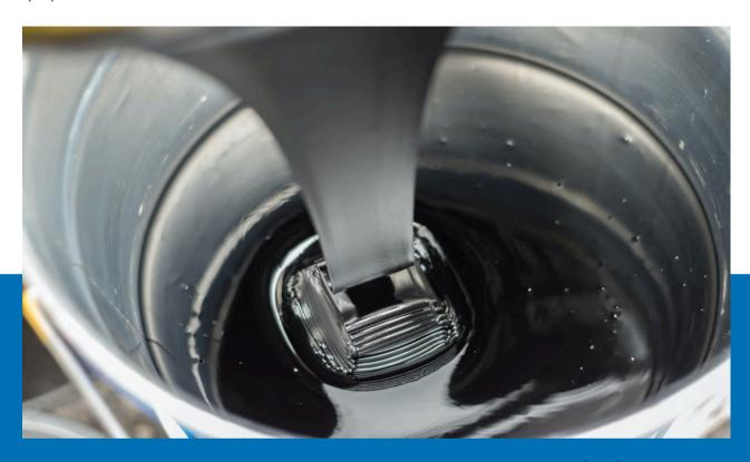
Performance Bitumen is used in the Production of **Polymer Modified Bitumen (PMB)**, which exhibits superior Properties such as increased Elasticity, improved Deformation Resistance, and enhanced fatigue Performance compared to conventional Bitumen. PMB is particularly effective in Mitigating Rutting and Cracking under Heavy Traffic Loads and Extreme weather conditions, thereby Extending the Lifespan of Roads and Reducing maintenance costs.
